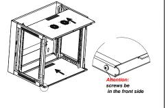
[5] Install top and bottom as shown by the arrow in the picture. Tip: Please note the direction when install bottom, screws will be in the front side,
